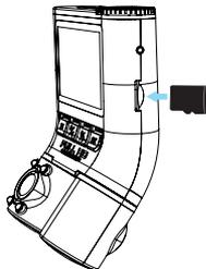
1. Insert a microSD card (minimum Class 10,16Gb) into the camera and push firmly until it locks into place.
