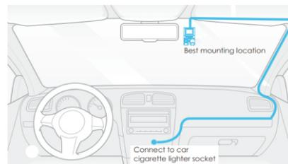
4. Wipe clean the chosen area of the windshield with a dry cloth; it must be completely grease free for the sticky pad to stick securely. Use detergent or an alcohol based wipe to remove any grease.
