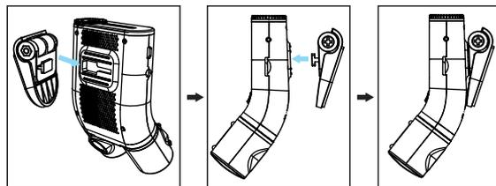
3. Select a location on the windshield, just a little below the rear-view mirror. The front lens needs to look through the area swept by the windshield wipers. The cabin lens needs to be able to see under the mirror, the camera can be placed alongside or behind the mirror. It should not obstruct the driver's view of the road.
