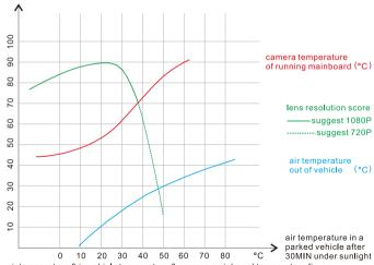
air temperature & in vehicle temperature & camera mainboard temperature figure
