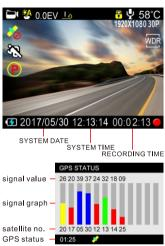
hold the OK button and power to active GPS TESTER
