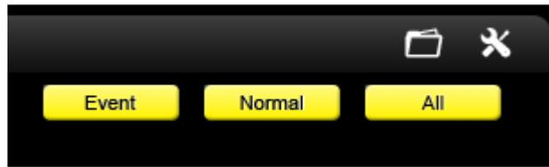
**EVENT:** will list only the files that have been created by the camera because of an EVENT. This could be a collision, a pothole or a manual event created by pressing the E button on the camera.
