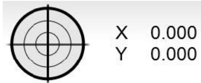
Below the main windows is a G-Force Meter display. The small spot in the centre of this meter represents the G-Force experienced by the camera at the time the video was recorded. As the vehicle accelerates you would expect to see the spot move towards the bottom of the meter. Braking will show up as the spot moving upwards on the meter. Cornering will send the spot left or right. The more heavy the manoeuvre, the further the spot will travel on the graph.
