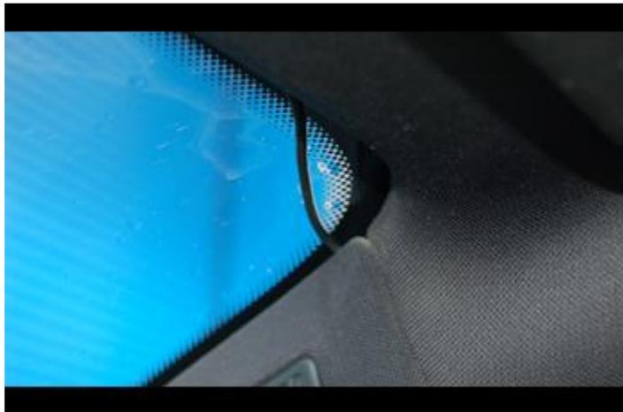
**7:** Attach the camera to the mount and face it forwards. Keep the camera as level as possible. (in a Truck or Bus, aim the camera slight down)
